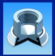
This device enables an elastomer to be used that offers higher mechanical performance. We have not forgotten the economic aspects; this concept is more compact, uses less material and is quicker to replace.
